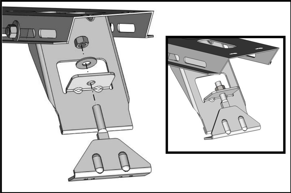
**Loosely** attach (4) **OUTER CLAMPS** at locations shown here using (4) 3/8 Flat Washers and (4) 3/8 E-Stop Nuts.
