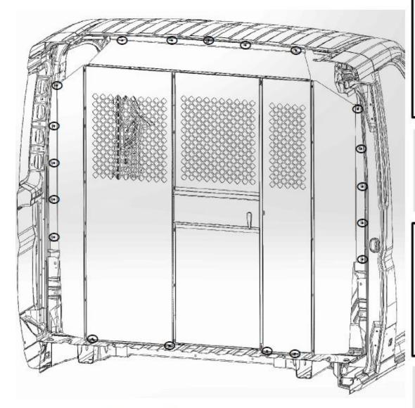
Torque Settings: 1/4-20 Grade 8 = 10 to 13.5 ft-lbs M6 Grade 10.9 - 11 to 15 N-m Standard Install: Mount the assembled partition to the installed Plusnuts\*.
