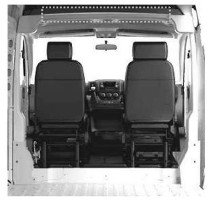
Locate the OEM hex-holes along the front Roof Bow (marked with a star in the above image), and install 5x Plusnuts\*.
