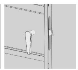
Snap the CAB-Side Door Handle into the hex cutout (be sure that lock cam is aligned properly). Secure the Cargo-Side Door Handle to the square rod protruding from the back of the Cab-Side Door Handle.
