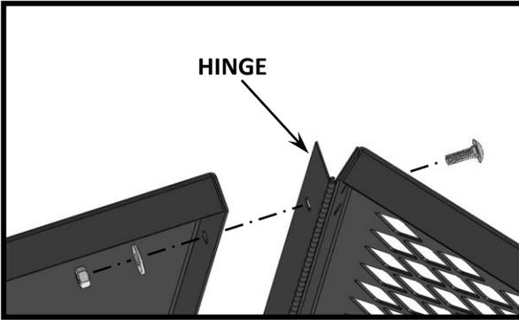
Align holes in Hinge on Door as shown and secure using:
