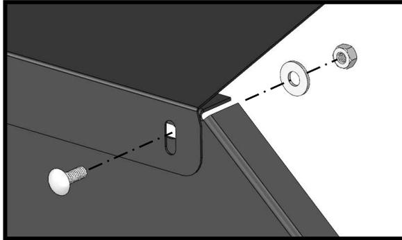
Align holes in Top Panel as shown and secure using:
