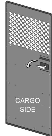
Once the handle is installed, turn clockwise to open from the outside, and counter clockwise to open from the inside.
