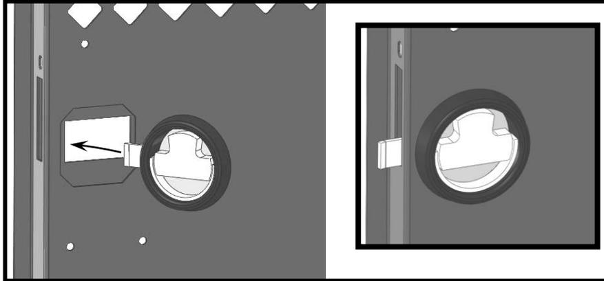
Insert the Round Handle into door cutout, so that the locking mechanism fits through the slot in the Center Panel. **NOTE: Be sure the Locking Mechanism is parallel to the floor before attaching the inside Handle.**
