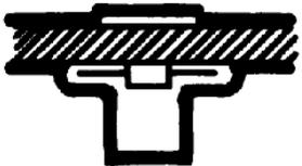
Fully upset Plusnut® provides a reliable nut plate for fastening.
