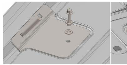
**Figure 9 Typical REAR adapter plate installation** *Note that carriage bolt is toward REAR of vehicle*
