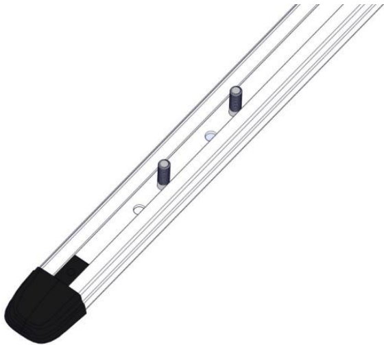
Step 7.1 Starting at the rear of the vehicle, use the 2nd hole as shown.
