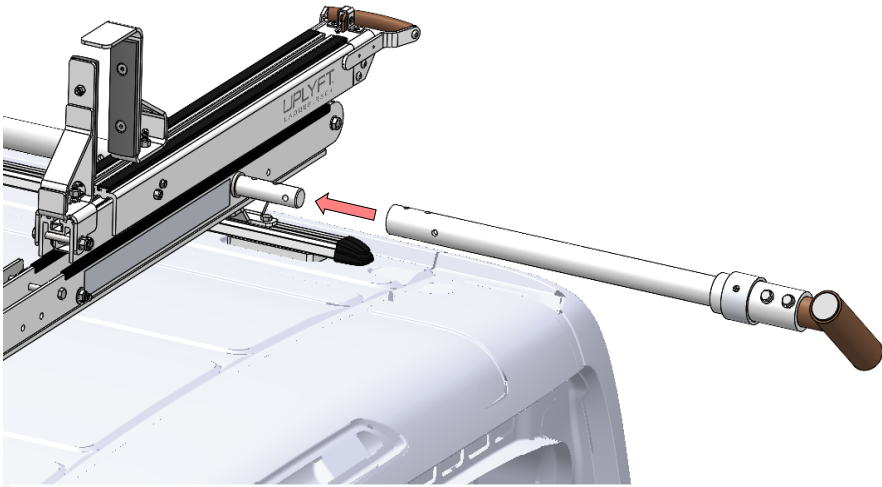
Step 19. Install and tighten the handle assembly Using a 1/2" wrench and 1/2" impact wrench, 5/16" x 2" bolts with the 5/16" washers and 5/16" lock nuts 02P168.
