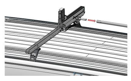
**Step 9.**Slide the front crossbow assembly into the connecting tube as shown.
