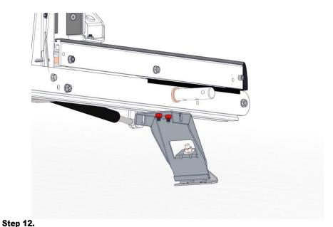
Using a 1/2" wrench, tighten the mounting brackets under the crossbow as shown.
