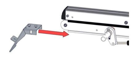
**Step 4.**Slide the mounting brackets into the crossbows as shown with the tabs facing
