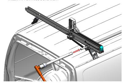
**Step 13.** Install the handle into the rear crossbow as shown.
