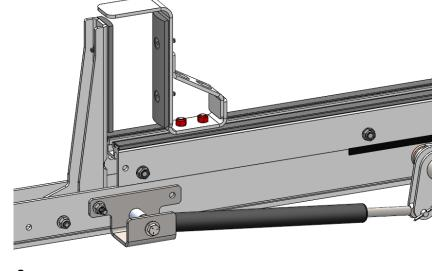
**Step 2.** Using a 1/2" wrench, tighten all the nuts as shown.
