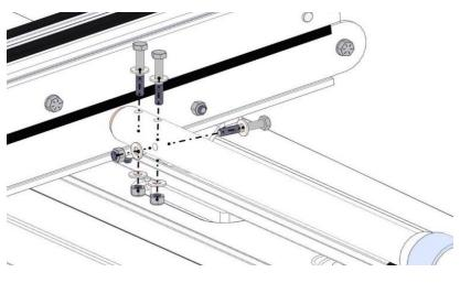
**Step 14.**Fasten handle with 5/16 X 2-1/2 bolts (3) and washers (6) and apply anti seize to bolts.
