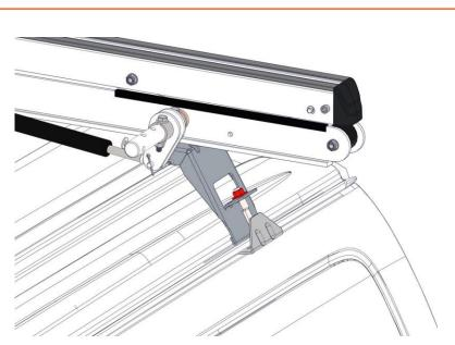
**Step 11.**Using a 9/16" wrench, tighten the front and rear crossbow mounts to the rain rail.
