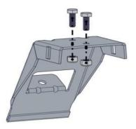
**Step 3.**Install the 7/8" bolts (02P394) through the main mounting brackets (02P816) and apply the nuts (02P168) on the bottom and finger tighten only.
