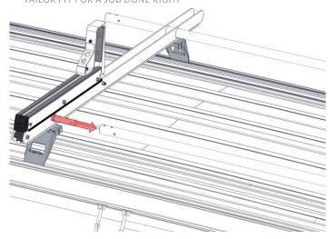
**Step 8.**Install middle crossbow through the long connecting tube, and into the short
