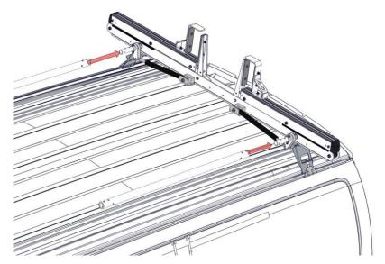
**Step 7.**Install the connecting tube (02P328) into the rear crossbow assembly.
