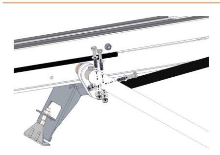
**Step 10.**Using a 1/2" wrench and 1/2" impact wrench, install and tighten the connecting tube 5/16" x 2" bolts (RM511497) with the 5/16" washers and 5/16" lock nuts (02P168).
