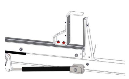
**Step 2.** Using a 9/16" wrench, tighten all the nuts as shown.
