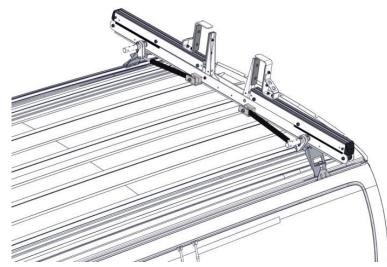
**Step 5.**Set the assembled rear crossbow on the vehicle as shown.
