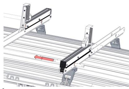
**Step 9.**Set the front crossbow in place and slide into the connecting tube
