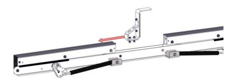
**Step 1.** Slide ladder stops (02P663) inside crossbows 4 per double rack and 2 per single rack.
