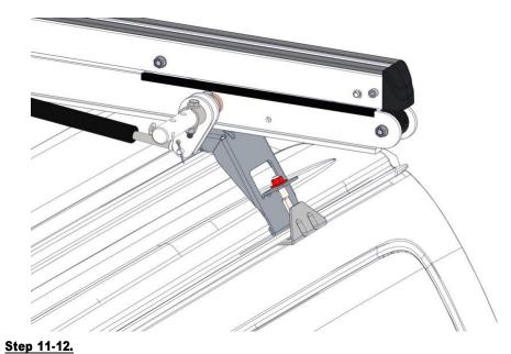
Using a 9/16" wrench, tighten the front and rear crossbow mounts to the rain rail.
