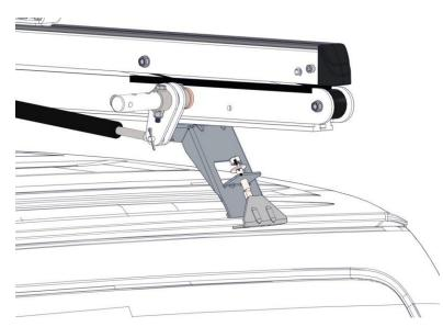
**Step 6.**Finger tighten the clamp assembly (M847010) with a 3/8" washer (RM541204) and 3/8" lock nut (02P168) as shown.
