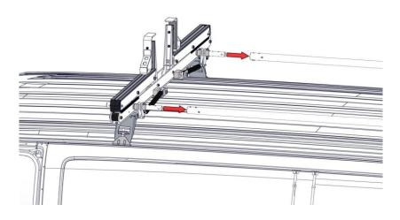
**Step 8.**Slide the front crossbow assembly into the connecting tube as shown.
