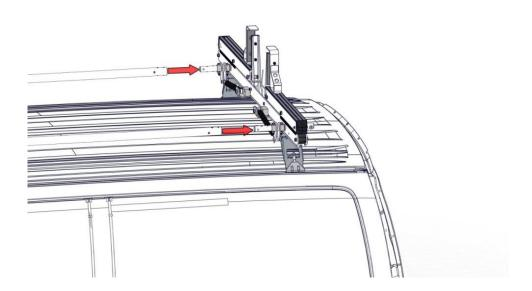
**Step 7.**Install the connecting tube (02P328) into the rear crossbow assembly.
