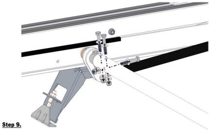
Using a 1/2" wrench and 1/2" impact wrench, install and tighten the connecting tube 5/16" x 2" bolts (RM511497) with the 5/16" washers and 5/16" lock nuts (02P168) and apply anti seize to the bolts.
