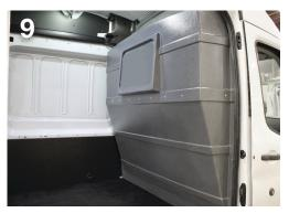
Adjust the weatherstripping along the door frames. The rubber should cover the outer edge of the panel. Installation is complete.
