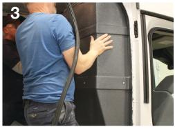
Slide the partition into place so that it lines up against the B-Pillar and along the headliner. Reattach the D-rings.
