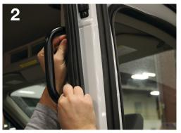
Pull back the weatherstripping around the door frame. Remove the pillar handle.
