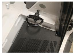
Remove the D-rings using a 1/2" nut driver.
