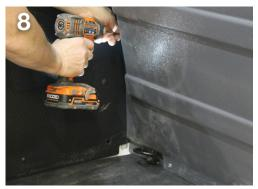
Loosely secure the sides and top of the partition with self-tapping screws (**E**), using the 1⁄4" nut driver, in the predrilled holes. When properly positioned, tighten all bolts.
