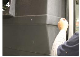
Mark the holes at the top of the partition, on the bottom bracket and in the partition at the end of the steel rib on the B-pillars. Remove the D-rings once more and remove the partition.
