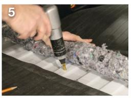
Drill the holes in the floor and B-pillar with the 11/32" drill bit. Insert the plus nuts (**A**), using the plus nut gun, in the 11/32" holes.
